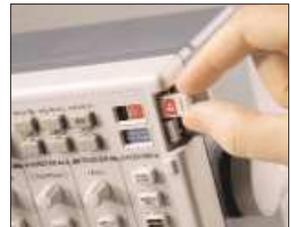
Application Module being installed.
