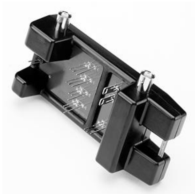
067-0405-00 TDS7000 series probe calibration and deskew fixture (front side).
